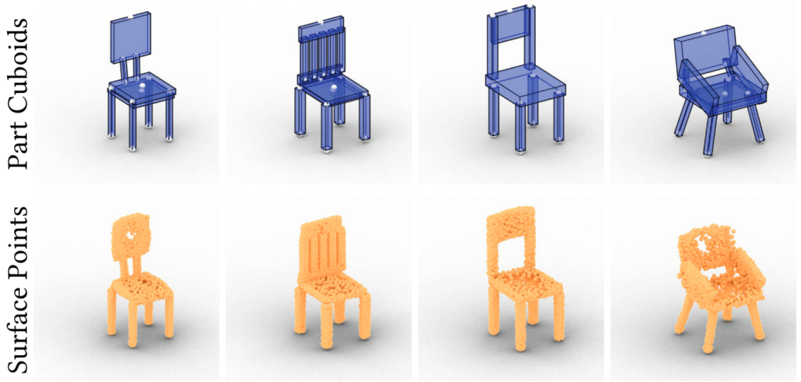
Figure 3.11: Converting generated SHAPEASSEMBLY programs into dense point clouds. We use a point cloud decoder to predict the surface geometry of each leaf part proxy in our 3D shape structure. In this process, geometric details begin to take form, at the cost of some artifacts. We discuss a method for improving this procedure in section 3.6.
